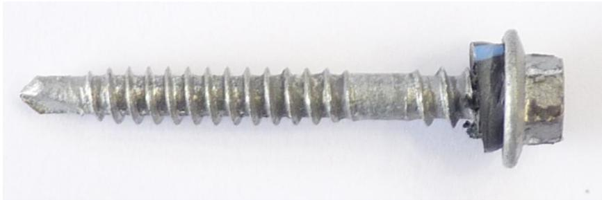
Figure 4. Tek screw used to fix cladding to timber framing. Measured overall length = 55 mm, 14 mm steel washer under hex head, 4.8 mm outside thread diameter
