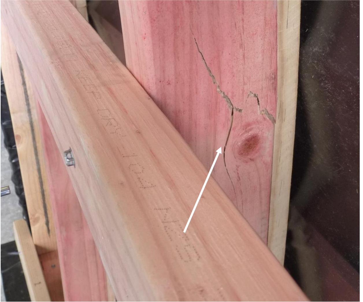
Figure 6. Failure of timber stud in Test 1
