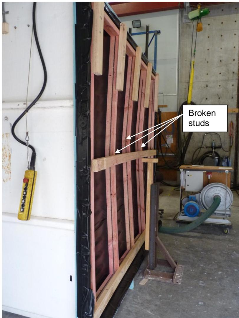
Figure 5. Failure of timber studs in Test 3.
