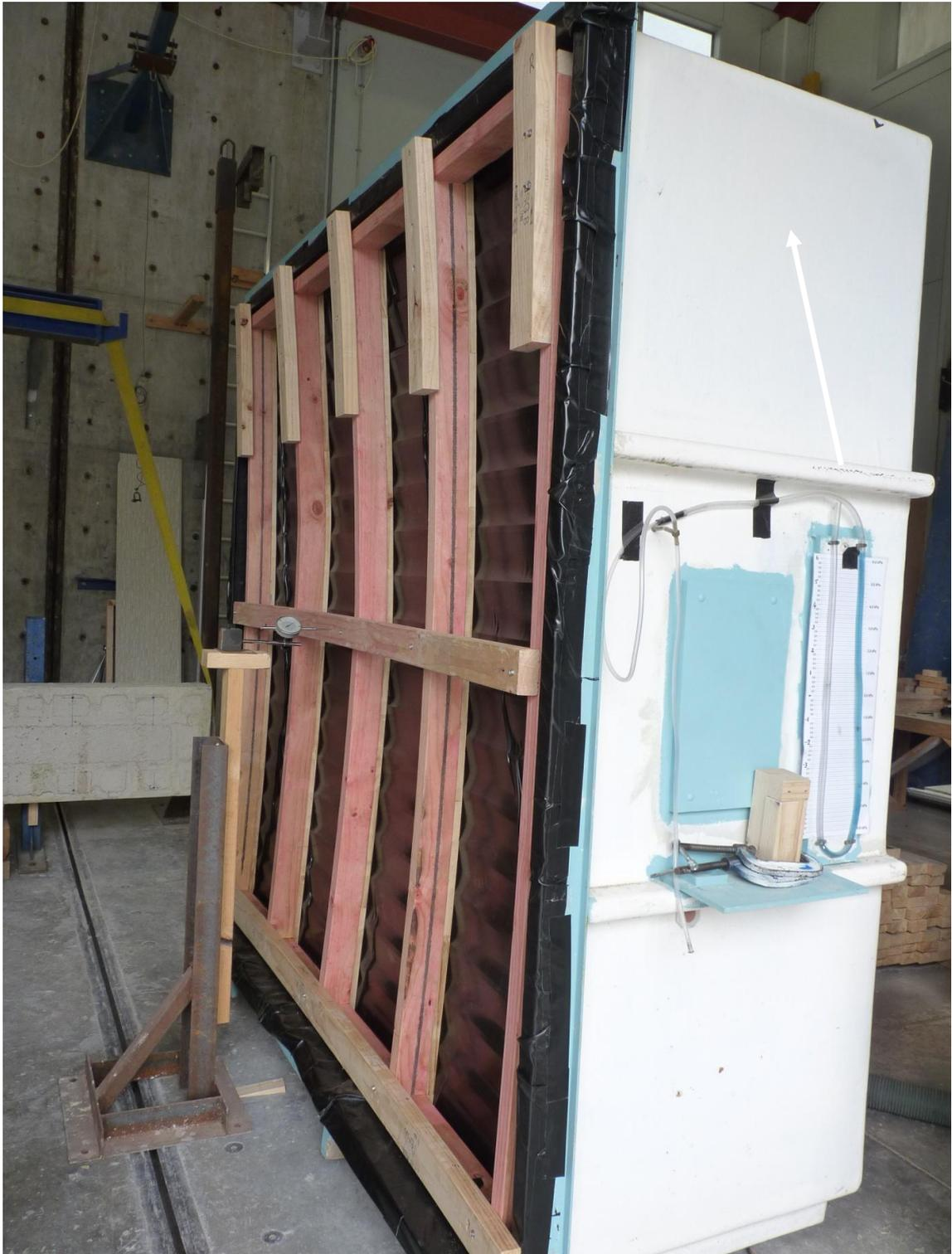
Figure 1. Test specimen in pressure box under high suction load. Note, curvature of studs.
