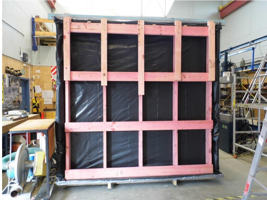
Figure 1. Eurobord Face Load Specimen Installed in Pressure Box
